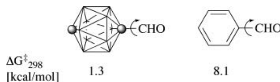
Figure 4. Calculated (MP2/6–316(d)) free energy of activation to internal rotation around the ring–CHO bond [17].
